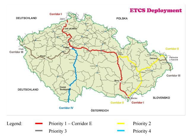
Fig. 7 – First phase of the ETCS Level 2 implementation
