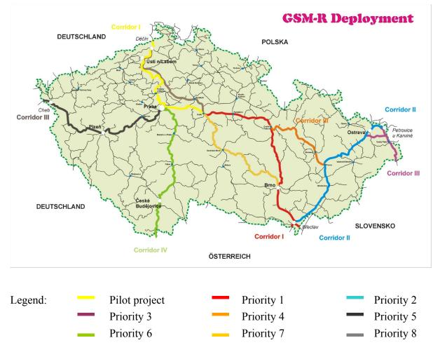
Fig. 5 – First phase of GSM-R implementation
