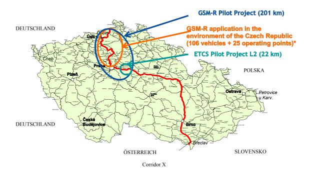
Fig. 3 – ERTMS/GSM-R, ETCS pilot projects and GSM-R application
